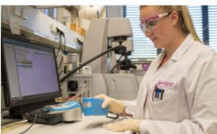
Katrin Basler checks the yellowness of a sample, evaluating PVC tarpaulins for roofs that have been exposed to the elements for nine months. Rain, sun, wind, dirt – all contribute to a natural stress test for these samples. Roofing membranes need to withstand all weather conditions for at least 20 years or longer. Therefore, Oxeno always tests the products under real outdoor conditions in addition to conducting artificial weathering in the laboratory.
