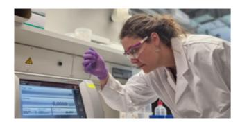
Here, Melike Beyram carries out a test to verify the viscosity of ELATUR® DINCD. This is used to determine the flow behavior of the product, as the viscosity of the plasticizer will always influence the customer's formulation.
