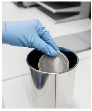
coarse activated carbon. These cans are then heated in an oven and the mass loss of the samples is measured by weighing them to determine the amount of volatile substances emitted. The metal cans enable rapid, multiple determination of the volatility values in the respective formulation while protecting the samples from strong air currents. The wire baskets act as spacers between the samples and the activated carbon to prevent the plasticizer from migrating into the carbon.
