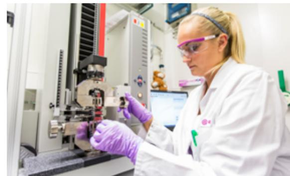
First, several tension rod samples are taken from the freely weathered specimen. The laboratory technician then clamps a tension rod into the testing to check the tensile strength and elongation at break. To ensure data accuracy, multiple tests are conducted. This process is repeated with new tension rods and the average values are analyzed. This rigorous testing provides application technology experts with a comprehensive understanding of the mechanical strength of ELATUR® DINCD.
