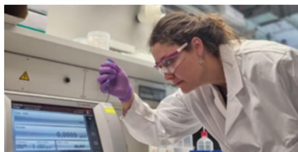
Here, Melike Beyram carries out a test to verify the viscosity of ELATUR® DINCD. This is used to determine the flow behavior of the product, as the viscosity of the plasticizer will always influence the customer's formulation.
